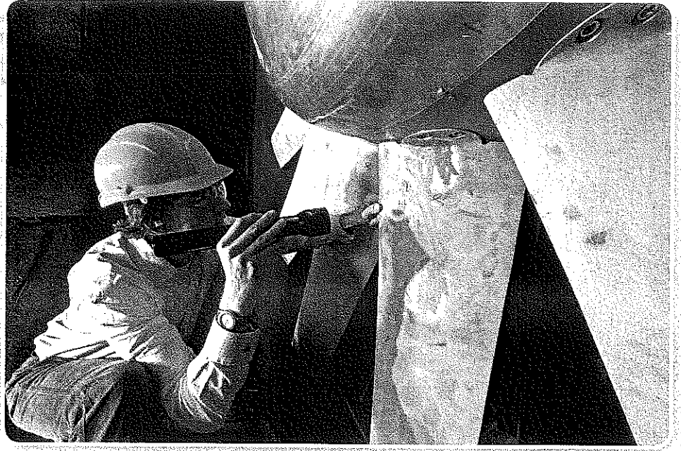
FIGURE 1-24: This aerospace engineer is inspecting the blades of an industrial wind tunnel.
